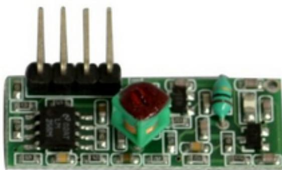
ZR-3A wireless Super regenerative radio receiver module 315MHZ 433.92MHZ 2mA wireless remote control 1 Receiver frequency: 315MHZ / 433.92MHZ 2 Operating voltage: DC 3V / 5V ± 0.3V 3 Operating current: 2mA 4. Demodulation mode: ASK 5 output data level: TTL level 6. Receiver sensitivity:-106dBm 7 Working temperature: -10 °C ~ +60 °C 8 Maximum dimensions: 30 \* 12 \* 10mm
